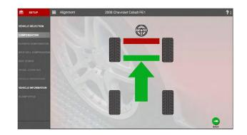
Once the vehicle has returned to the start position, compensation is complete. If changes were detected in one or more suspension angles the screen will alert the user to roll the vehicle to relieve stress and then to perform compensation again. Click Next to continue.
