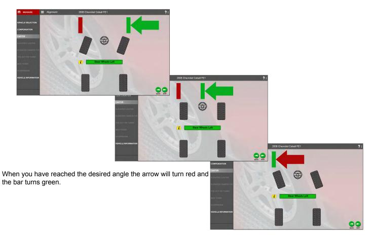
Steer back to center. When the wheels are centered the position bar turns to green and the direction arrow will turn red to indicate correct position.
