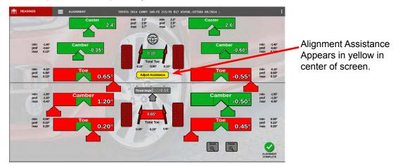
Specifications for the vehicle under test are shown on the screen with minimum, maximum and preferred values. The actual live value is shown inside the measurement block. Cross values, total toe and thrust angle are displayed in the center of the screen.
